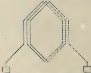
FIG. 177.—Two-circuit Winding— three-turn coil.
